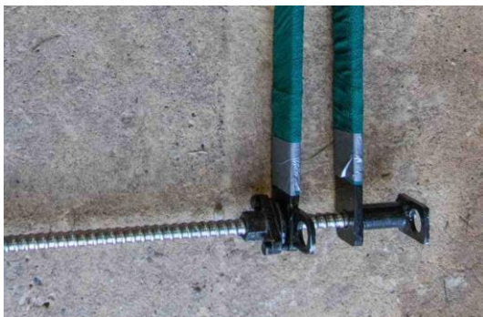
Figure 4. Steel tie rod (used for scaffoldings)
