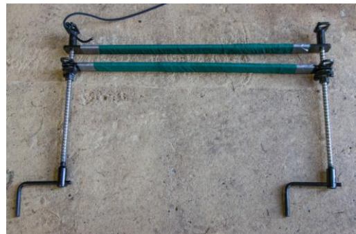
Figure 3. Type 2 elephant mouth opener (gag), pushing the lower mouth piece down, including 2 fixed handles.
