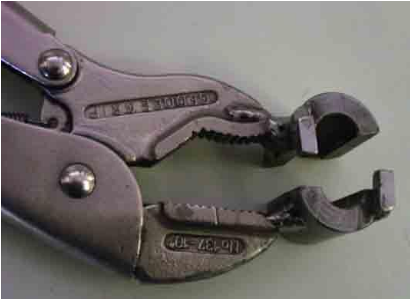
Grip plyer with custom made mouth piece to cut syringe perpendicular
