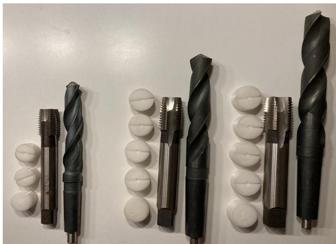
Figure 7. Nylon threaded rods, thread makers and drills in various sizes. © Willem Schaftenaar.
